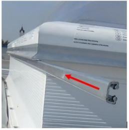
Fig. 40. Lubricating the hinge.
